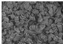
Figure 6: Scanning Electron Microscope (SEM) image of clay surface, where the dark regions indicate the presence of water (source: minersoc.org)
